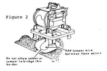
More than one antenna port can be "picked up"at one time by applying control voltage to more than one relay at one time. This allows the user considerable flexibility in stacking arrays of similar antennas.
