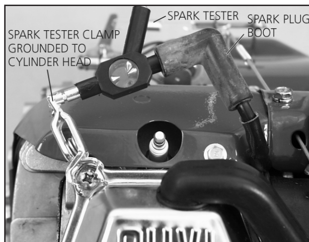
Figure 8.5 — Testing Ignition System
