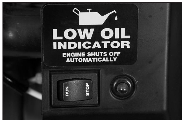
Figure 12.14 — Low Oil Indicator
