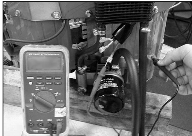
Figure 7-2. Testing DC Output Wire
