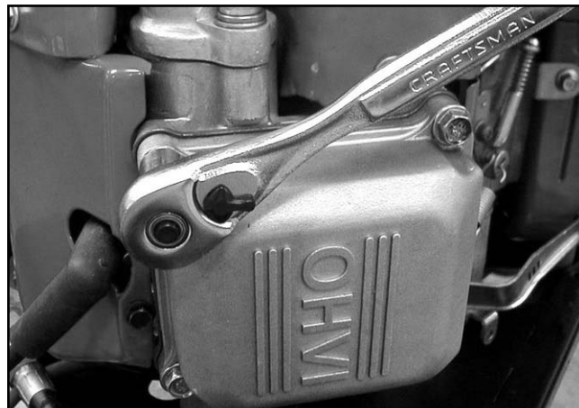
Figure 13-16. Install Valve Covers
