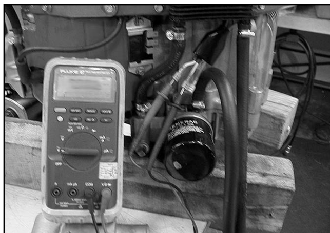
Figure 7-1. Testing AC Output
