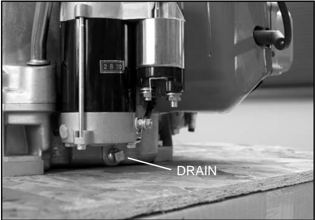
Figure 8-3. Oil Drain Location
