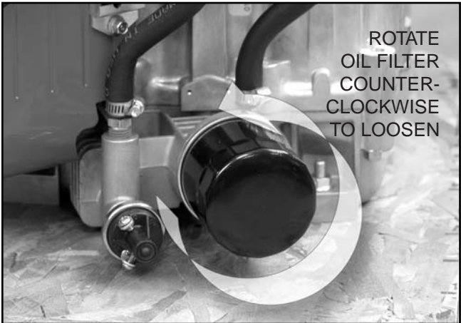
Figure 8-4. Removal of Oil Filter
