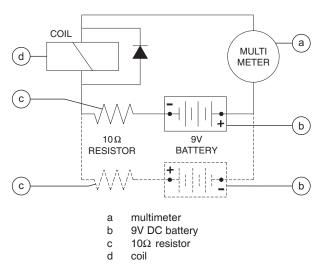
Note: Dotted lines in illustration indicate a reversed connection as specified in step 6
