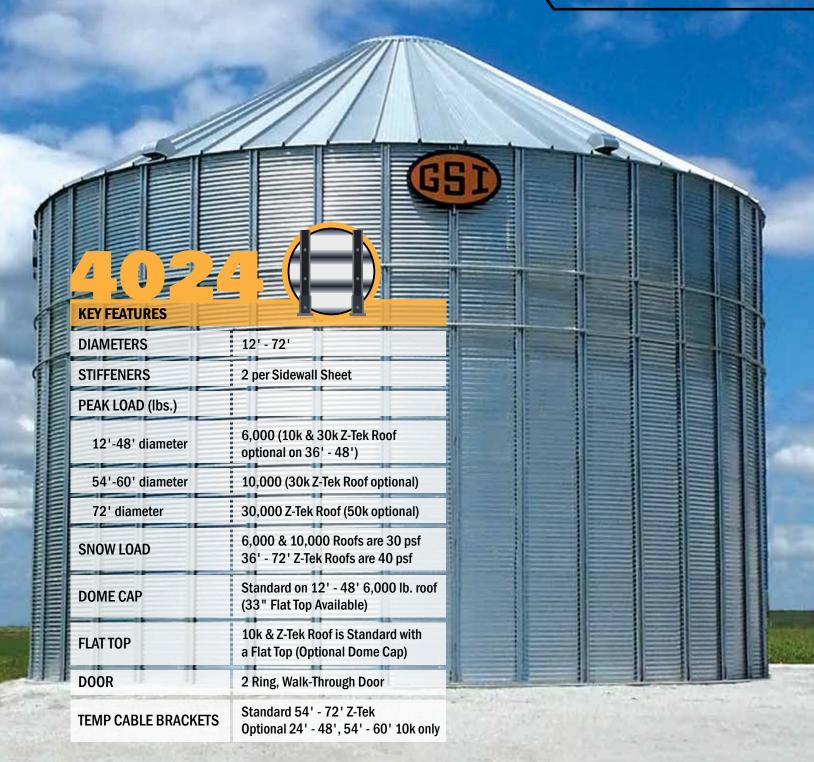
GSI stiffened bins use vertical stiffeners to channel the load of the bin to the foundation more effectively. With storage capacities from 1,000 bushels up to 1.2 million bushels, these bins are designed to expand with you as your operation grows. One of GSI's newest bin offerings, the 4024, features 4" corrugation and storage capacity over 280,000 bushels – the ideal solution for commercial operators faced with growing storage needs.
