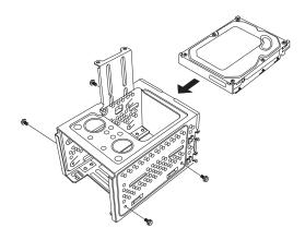
3 Place the hard disk drive cage into the chassis. The two screw holes on the hard disk drive cage (A) should be aligned with the screw holes on the chassis (B).
