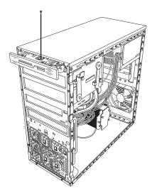
3 Disconnect the cable from the back of the memory card reader.
