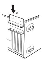
4 Inside the PC, locate the add-in card slots on the motherboard.
