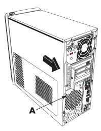
3 Use the handle to pull and slide the panel back about 1 inch (2.5 centimeters), and then lift it off the chassis.
