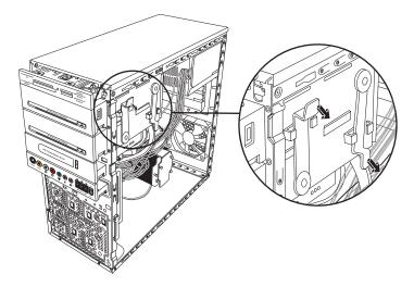
**6** Connect the power and data cables from the back of the optical drive you want to add. Reconnect the sound cable, if present.
