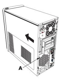
**NOTE:** There is a 3mm gap between the top of the side panel and the top of the chassis when the side panel is attached properly.
