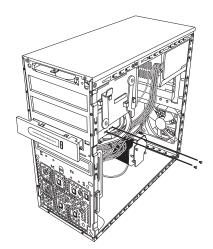
3 Disconnect the power and data cables from the back of the drive by squeezing the two latches and pulling the cable.
