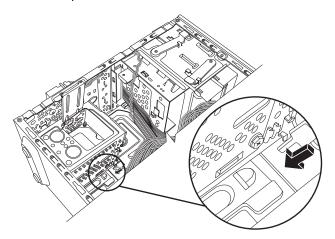
5 Attach the hard disk drive cables.
