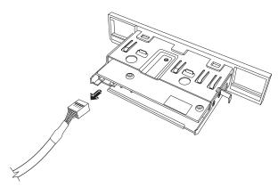
4 Pull the memory card reader out of the front of the chassis.
