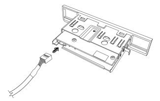
4 Push the memory card reader into the chassis until the screw hole on the chassis is aligned with the screw hole on the top of the memory card reader, and then insert the short screw to secure the memory card reader to the chassis.
