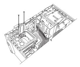
7 Complete the procedures to replace the front panel, replace the side panel, and close the PC. See "Opening and Closing the PC" on page 1.
