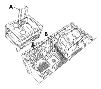
4 Align the four guides on the bottom of the hard disk drive cage with the holes on the back of the chassis, and then slide it down toward the bottom of the chassis until it locks into place.
