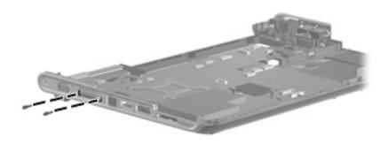
Where used: Two slotted screws that secure the system board to the base enclosure
