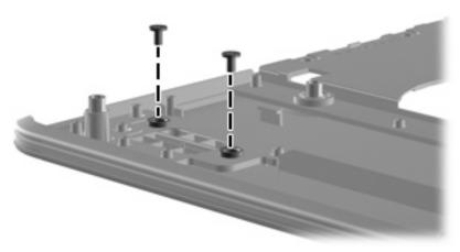
Where used: Two broadhead screws that secure the fingerprint reader board to the top cover
