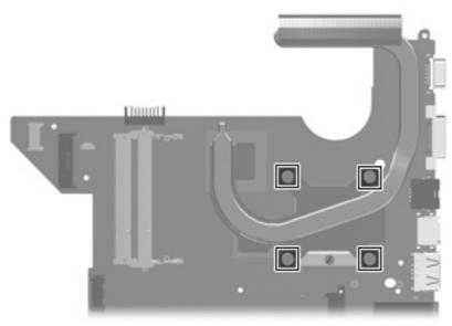
Where used: Four captive screws (secured by C-clips) that secure the heat sink assembly to the system board
