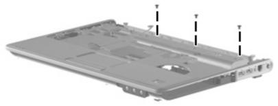
Where used: Three screws that secure the top cover to the computer
