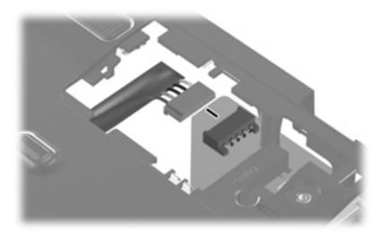
3. Remove the two Phillips PM1.5×9.0 slotted screws (1), and the Phillips PM2.5×4.0 screw (2) that secure the system board to the computer.
