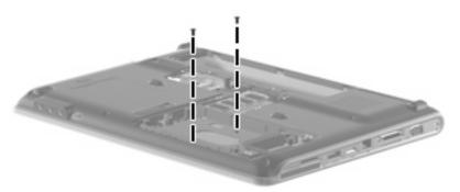
Where used: Two screws that secure the top cover to the computer
