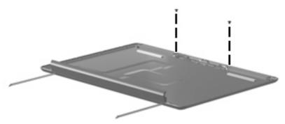
Where used: Two screws that secure the wireless antenna transceivers to the display enclosure
