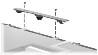
Where used: Two screws that secure the camera/microphone module to the Flush Glass display assembly
