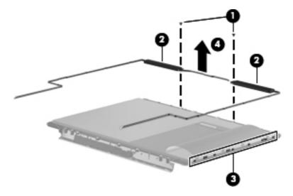
Reverse this procedure to reassemble and install the Flush Glass display assembly.
