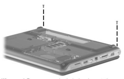
Where used: Two screws securing the keyboard cover to the computer
