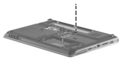
Where used: One screw that secures the top cover to the computer
