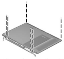
Where used: Six screws that secure the hinge to the Flush Glass display assembly
