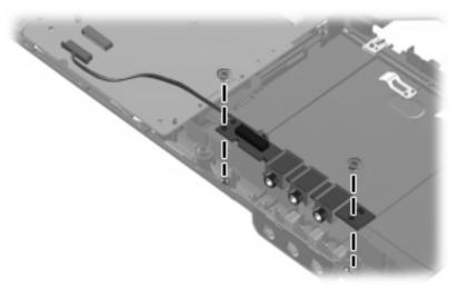
Where used: Two screws that secure the audio board to the computer
