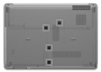
Where used: Four captive screws that secure the hard drive, memory, and WWAN covers to the computer
