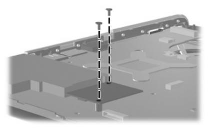
Where used: Two screws that secure the modem module to the computer
