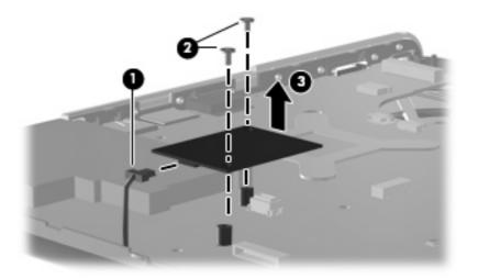
Remove the modem module.
