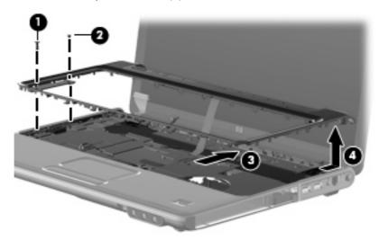
Reverse this procedure to install the keyboard cover.
