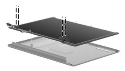
Where used: Four screws that secure the display panel to the display assembly
