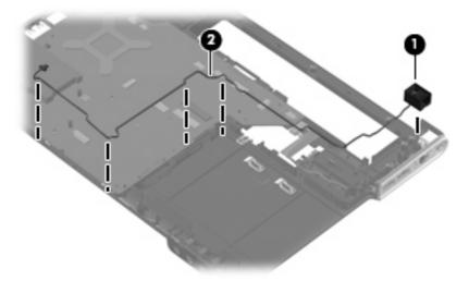
Reverse the preceding procedure to install the modem module cable.
