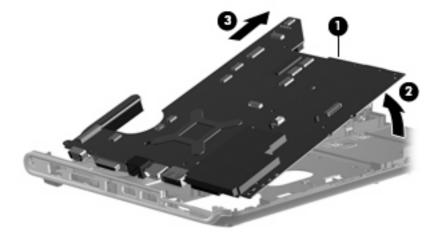
When replacing the system board, be sure that the following components are removed from the defective system board and installed on the replacement system board:
