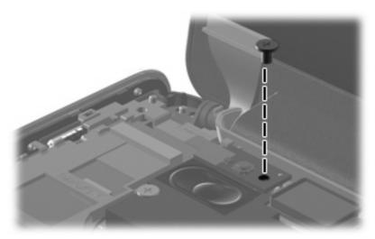
Where used: One screw that secures the power button board to the computer
