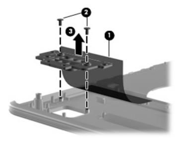
Reverse the above procedure to reassemble and install the fingerprint reader.
