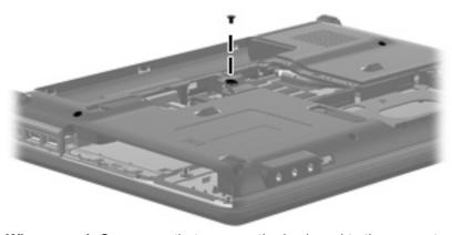
Where used: One screw that secures the keyboard to the computer
