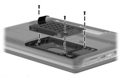
Where used: Three screws that secure the hard drive to the computer
