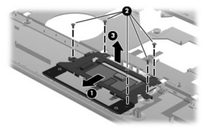
Reverse the above procedure to reassemble and install the TouchPad.
