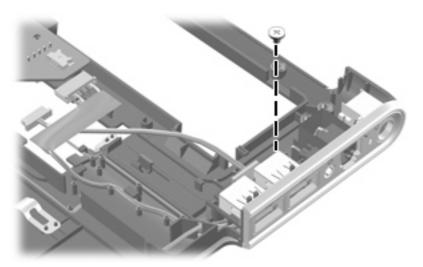
Where used: One screw that secures the USB board to the computer
