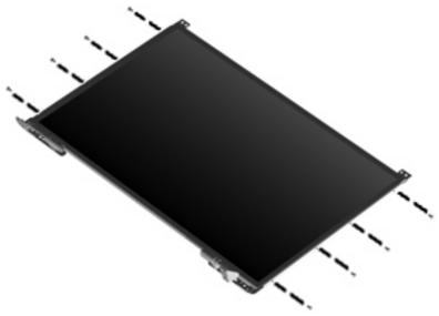
Where used: Eight screws that secure the display assembly hinge to the computer
