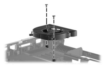
Where used: Two screws that secure the fan to the system board
