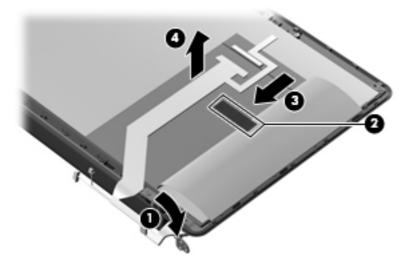
13. If it is necessary to replace the inverter, remove the four Phillips PM2.5×4.0 screws (1) that secure the inverter cover to the display assembly, and remove the inverter cover (2).
