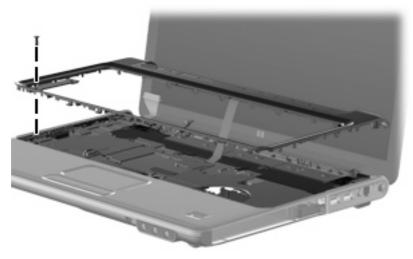
Where used: One screw that secures the keyboard cover to the top cover
