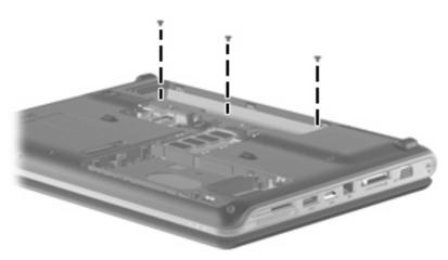
Where used: Three screws that secure the keyboard cover to the computer
