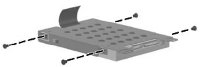
Where used: Four screws that secure the hard drive bracket to the hard drive
