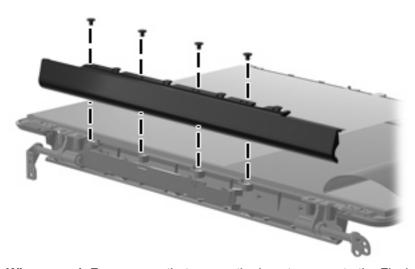
Where used: Four screws that secure the inverter cover to the Flush Glass display assembly
