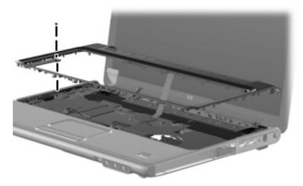
Where used: One screw that secures the keyboard cover to the top cover
