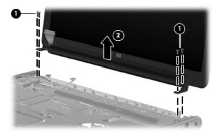
If it is necessary to replace other display assembly components, continue to the section that corresponds to the appropriate display assembly
