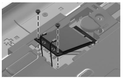
Where used: Two screws that secure the WWAN module to the computer
