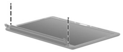
Where used: Two screws that secure the bezel to the display assembly
