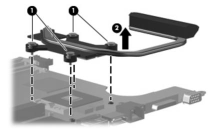
NOTE: Each time the fan and heat sink are removed, the thermal material must be thoroughly cleaned from the surfaces of the heat sink and system board components: heat sink (1), processor (2), Northbridge clip (3), and capacitor (4). Thermal pads and thermal paste must be installed on all surfaces before the fan and heat sink are reinstalled. Thermal pads and thermal paste are included with all fan, heat sink, system board, and processor spare part kits.
