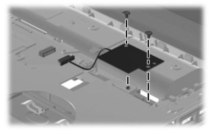
Where used: Two screws that secure the SIM connector board to the system board
