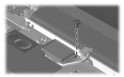
Where used: One screw that secures the Bluetooth module to the computer
