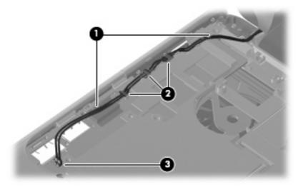
3. Remove the wireless antenna cable from the path (1) and disconnect it from the system board (2).
