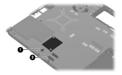
2. Disconnect the power connector cable from the system board.
