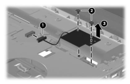
Reverse this procedure to install the SIM connector board.
