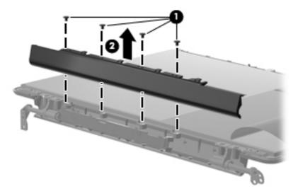
**14.** Release the inverter from the display assembly, and lift as far as the attached cables will allow **(1)**.
