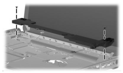
Where used: Two screws that secure the speaker assembly to the computer
