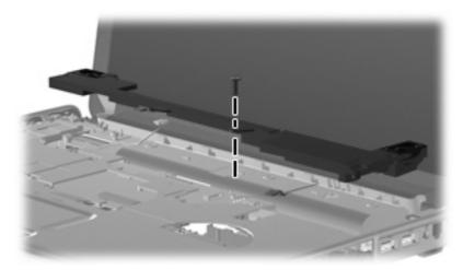
Where used: One screw that secures the speaker assembly to the top cover
