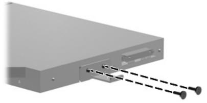
Where used: Two screws that secure the optical drive to the computer
