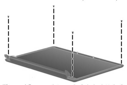
Where used: Four screws that secure the display bracket to the display assembly
