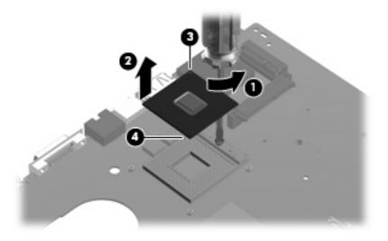
Reverse this procedure to install the processor.
