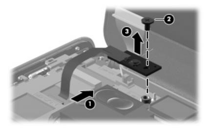
Reverse this procedure to install the power button board.
