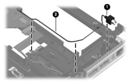
Reverse this procedure to install the TV tuner antenna cable.
