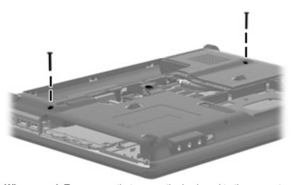
Where used: Two screws that secure the keyboard to the computer
