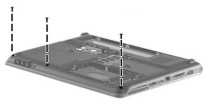
Where used: Three screws that secure the top cover to the computer
