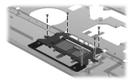
Where used: Five screws that secure the TouchPad to the top cover
