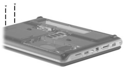
Where used: Two screws that secure the keyboard cover to the computer
