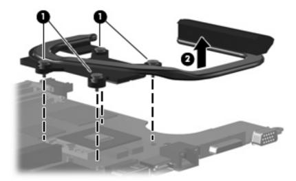
NOTE: Each time the fan and heat sink are removed, the thermal material must be thoroughly cleaned from the surfaces of the heat sink and system board components: heat sink (1), processor (2), heat sink (3), Northbridge clip (4), nVidia video chip (5), and capacitors (6). Thermal pads and thermal paste must be installed on all surfaces before the fan and heat sink are reinstalled. Thermal pads and thermal paste are included with all fan, heat sink, system board, and processor spare part kits.
