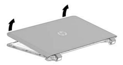
Turn the display with the bezel down and the back of the panel up. Disconnect the display cables from the panel and bezel(1), (2). Release the connections (3), (4) and lift the panel (5).
