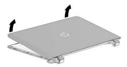
**b.** Turn the display with the bezel down and the back of the panel up. Disconnect the display cables from the panel and bezel(1), (2). Release the connections (3), (4) and lift the panel (5).
