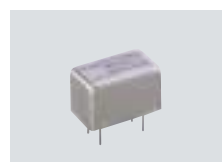
CR-338 HIGH STABILITY CRYSTAL UNIT Contains a temp. compensating heater for improved frequency stability. Frequency stability: ±0.5 ppm
