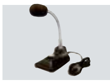
SM-6 DESKTOP MICROPHONE Electret condenser-type desktop microphone.
