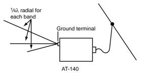
$^{1}\!/_{\lambda}$  (quarter wavelength) radial for each band is suitable for a counterpoise. Install the counterpoise directly below the AT-140's ground terminal. Insulate the ends of each radial from other metal objects. Layout the radial horizontally and as straight as possible.
