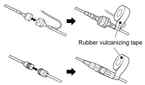
③ Fix both of the coaxial and control cables to protect the inside connections.
