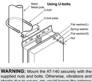
shocks due to waves, etc. could loosen the antenna tuner making if fall, causing personal injury.
