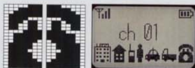
8x20 dot character can be made on a PC and plural characters can be combined on LCD.
