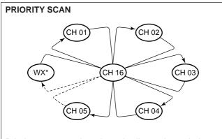
Priority scan searches through all tag channels in sequence while monitoring channel 16. When a signal is detected on channel 16, scan pauses until the signal disappears; when a signal is detected on a channel other than channel 16, scan becomes dualwatch until the signal disappears. Set the tag channels (scanned channel) before scanning. Clear the tag channels which inconveniently stop scanning, such as digital communication use.
