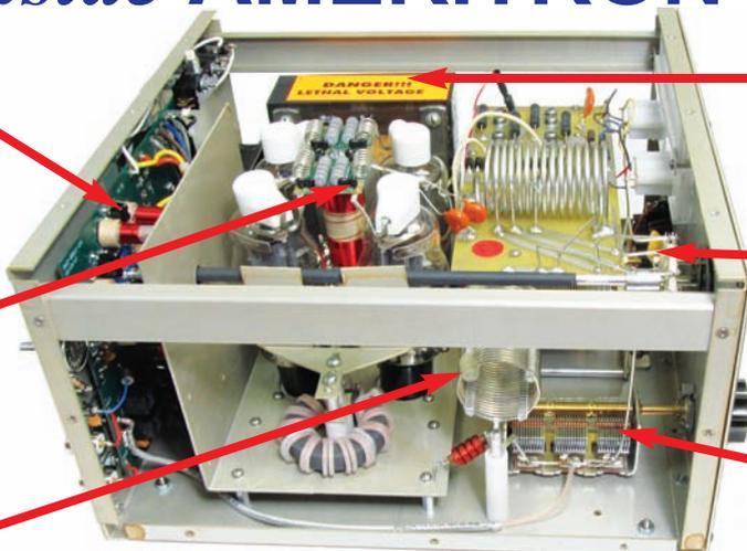
Heavy duty power supply: 17 lb. high silicone steel transformer and computer grade capacitors.
