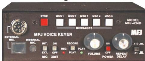
by your VOX PTT line. A closure to ground via remote control or computer also halts messages.
