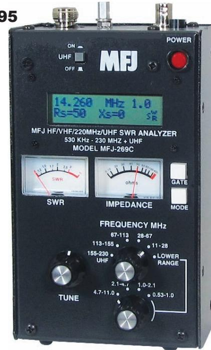
yagis, quads and other antennas and determine their SWR, resonant frequency and bandwidth.
