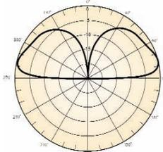
The R-8 AND R9 provide 360 degree (omni) coverage on the horizon and a low radiation angle in the vertical plane for a better DX.
