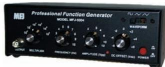
Gives precision sine, square and triangular wave forms from 1 Hz to 1 MHz in 6 decade ranges. Amplitude adjustable 0-12 volts peak-to-peak. DC offset is adjustable -6 to +6 VDC. Output is short circuit protected with output impedance of 400 Ohms. Sturdy black all metal cabinet. 110 VAC.
