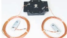
**MFJ-2012 Power-Lite™** 40/20/10/6 Meters, handles 1500 Watts PEP CW/SSB. 67' long overall, long leg 44.6, short leg is 22.5 feet. Robust high-power version of the MFJ-2010 with 14-gauge stranded-copper wire and porcelain end insulators. Pull-tested to 200 pounds.
