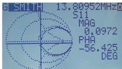
Smith Chart plot. Moveable cross-hair tracks plot over any frequency span. Displays S11 magnitude, phase angle at any frequency.
