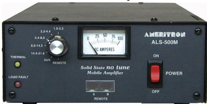
bypasses amplifier for "barefoot" operation. Extremely quiet fan comes on as needed. Excellent harmonic suppression, push-pull output, DC current meter. 13.8 VDC/80 Amps. Super-compact 3 1/2"x9"x15 inches. 7 pounds.
