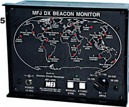
When each beacon completes a transmission it goes silent on that band and switches to the next higher band.
