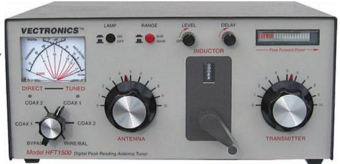
Antenna selector switch is a 6-position ceramic. Coax 1 is for tuned and tuner bypass; Coax 2 is for tuned and tuner bypass, bypass and balanced antenna.
