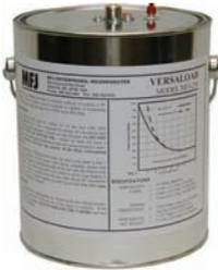
VersaLoad™ kW dummy load lets you run 1KW CW or 2 KW PEP for 10 minutes. Run 1/2 KW CW or 1 KW PEP for 20 minutes. Run continuous duty 200W CW or 400 W PEP. Derating curve. Quality 50 ohm non-inductive resistor.
