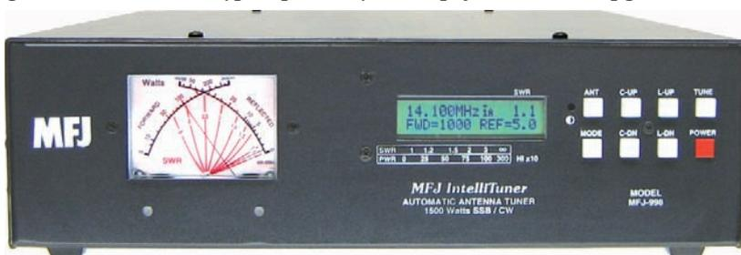
MFJ-998 is the smallest full legal-limit automatic antenna tuner in the world! 13Wx4Hx15D inches fits easily into your ham station. Weighs just 8 pounds -- great portability! Requires 12-15VDC at 1.4 amps maximum or 110 VAC with MFJ-1316, \$21.95.
