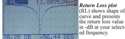
Return Loss plot (RL) shows shape of curve and presents the return loss value in -dB at your selected frequency.
