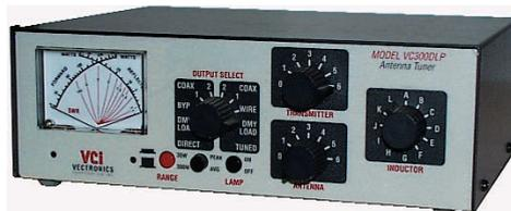
Has 4:1 balun for balanced line antennas. Handles up to 300 Watts SSB PEP, 200W continuous (150W, 1.8 MHz).
