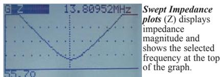
Swept Impedance plots (Z) displays impedance magnitude and shows the selected frequency at the top of the graph.
