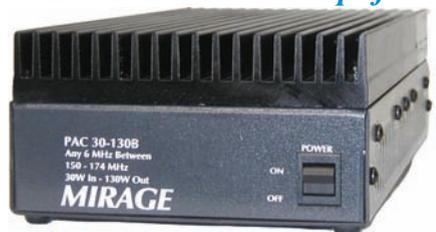
Commercial Amplifiers are available for 150-174, 450-470 MHz and VHF marine bands, 70-100 Watts out. Most feature over-temperature sensing that bypasses amplifier when safe operating temperatures are exceeded; heavy duty heatsinks finned on 3 sides; and wide input power range. These amps were designed for two-way radio signal commercial, mobile, or fixed location use. All are FCC type accepted.
