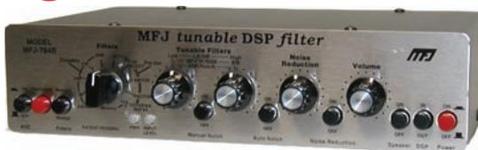
For example, tune one to mark, one to space and set bandwidth tight for a super sharp RTTY filter.
