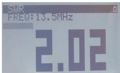
Single Frequency Mode. First screen shows SWR in BIG 3/4 inch digits and the Frequency reading in a single glance.
