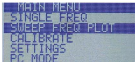
Main Menu selects these modes: Single Frequency, Swept Frequency, Calibration Screen (manages OSL calibrations), Settings Screen (basic analyzer setup) and PC Mode (dumps data in computer).
