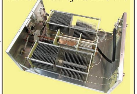
The MFJ-976 is a 1500Watt full Legal Limit fully balanced antenna tuner.
