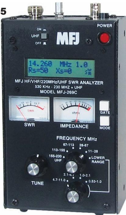
yagis, quads and other antennas and determine their SWR, resonant frequency and bandwidth.
