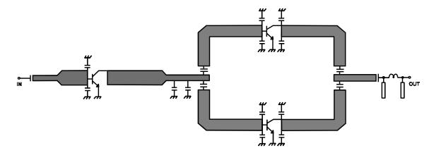
The input signal from the driver transceiver is matched to the base of the PAC 15-100-C driver transistor via a microstripline matching network. The collector of this stage is impedance at this point where the signal is split for amplification by twin power amp stages.
