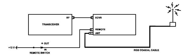
No tune-up should be required as the circuit is broad-banded to cover the entire 450-475 MHz band. If tuning is required, refer to the factor for service. Only a qualified holder of an FCC second-class radiotelephone license (or higher) should tune or otherwise adjust this amplifier. Additionally, a spectrum analyzer should be used to monitor harmonic and spurious outputs to ensure that proper operation is obtained.
