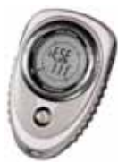
Brunton Nomad V2 Digital Compass Resolution: 1° Accuracy: ±2°
