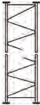
Bracing Detail for Sections 1W - 3WN Solid Round Legs & Solid Round Braces
