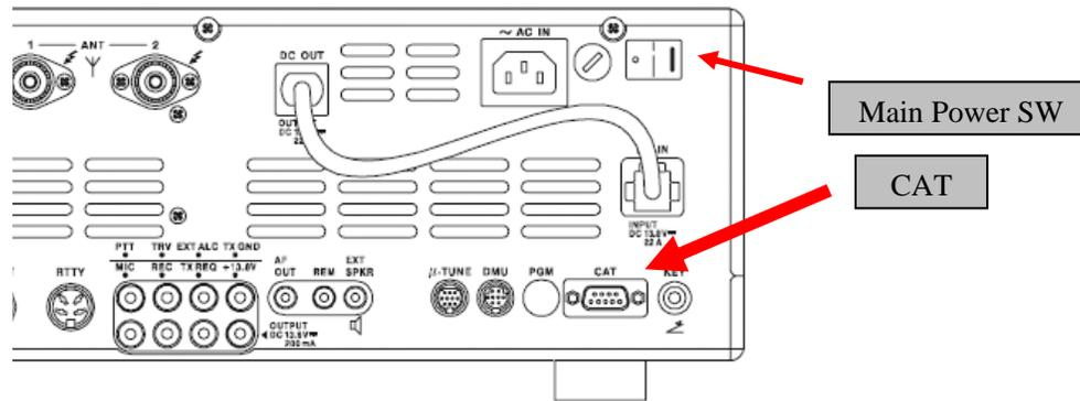
3. Reconnect the power cable and turn ON the main power switch located on the back of the FT-2000 (or turn ON the power supply for FT-2000D).
