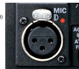
●Cannon (XLR) Connector (w/48V Mic Power LED engaged)
