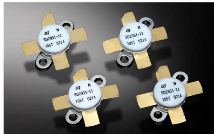
● 4 x 2SD2931 MOS FET Devices Produce 400 W of Output Power
