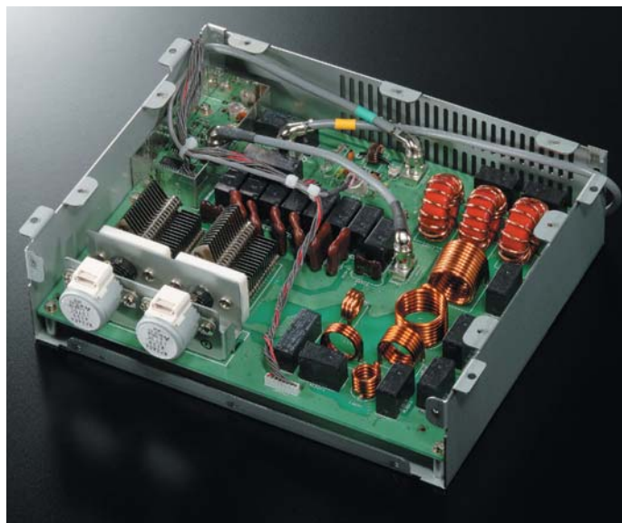
●Automatic, High-Speed 500-Watt-Capable Antenna Tuner
